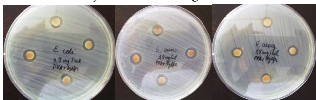
Figure 2. Testing the bactericidal activity of PVA/AgNps hybrid material to control bacterial strains by DDM.
