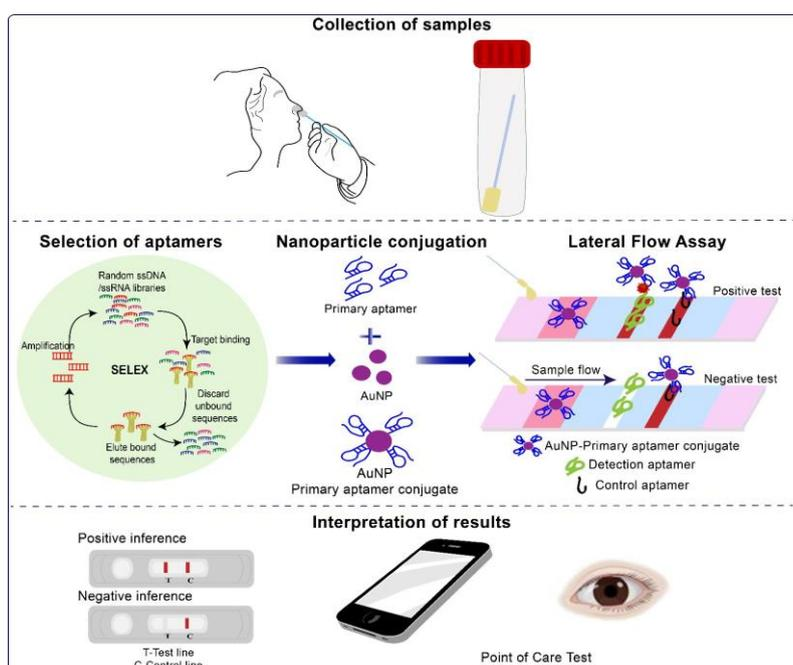
**Scheme 4.** Schematic illustration of designing and testing of aptasensor as a POCT device.
