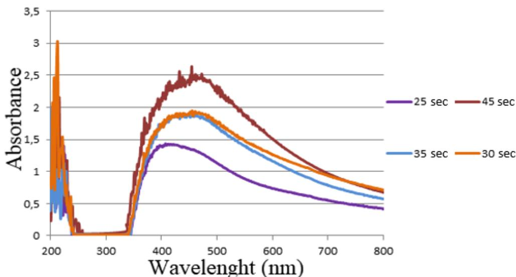
**Figure 2.** UV-Vis analysis of the green synthesis of AgNPs by different routes and different heating time variations.
