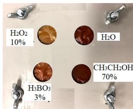
**Figure 6.** Feasibility test after 24 hours of contact with H<sub>2</sub>O, H<sub>2</sub>O<sub>2</sub>, H<sub>3</sub>BO<sub>3</sub>, and CH<sub>3</sub>CH<sub>2</sub>OH.
