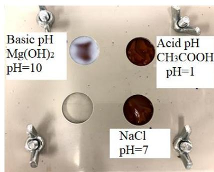
**Figure 7.** Feasibility test after 24 hours of contact with NaCl, Mg(OH)<sub>2</sub>, and CH<sub>3</sub>COOH solutions.
