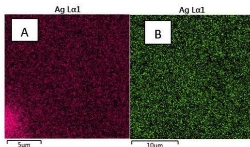
**Figure 11.** X-ray mapping images of the blend treated with NaCl (A) and CH<sub>3</sub>COOH, where the luminous dots represent the presence of Ag (B).
