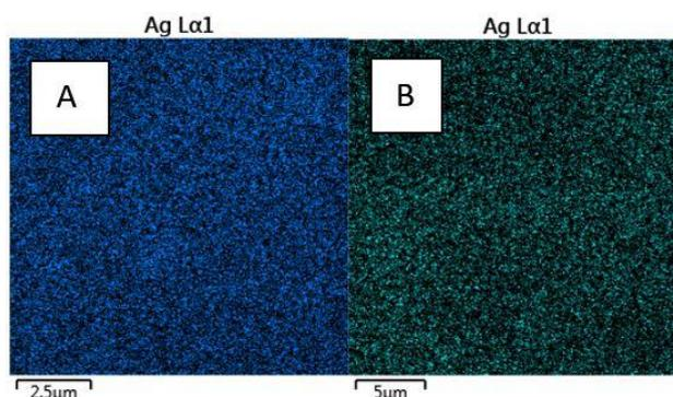
**Figure 13.** X-ray mapping images of the blend treated with CH<sub>3</sub>CH<sub>2</sub>OH (A) and H<sub>3</sub>BO<sub>3</sub> (B), where the luminous dots represent the presence of Ag.
