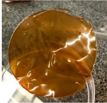
**Figure 3.** Biodegradable film synthesized by an extract with AgNPs.
