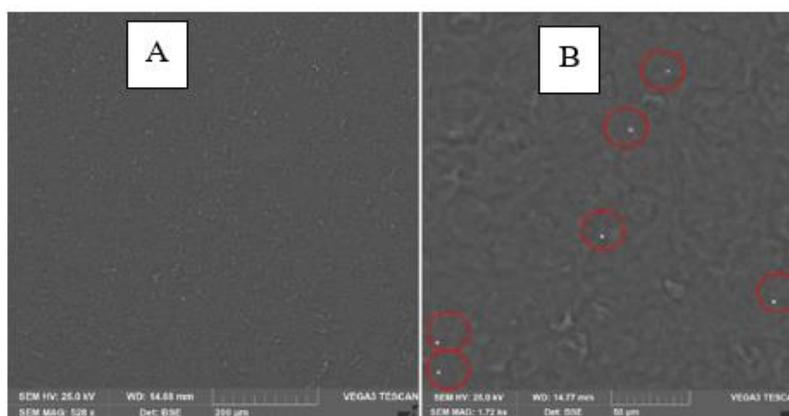
**Figure 9.** SEM micrographs of film III. In (A) 200 μm magnification and (B) 50 μm magnification with AgNPs marked in red circles.
