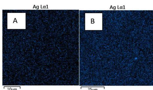
**Figure 12.** Images of X-ray mapping of the blend treated with Mg(OH)<sub>2</sub> (A) and H<sub>2</sub>O<sub>2</sub> (B), where the luminous dots represent the presence of Ag.
