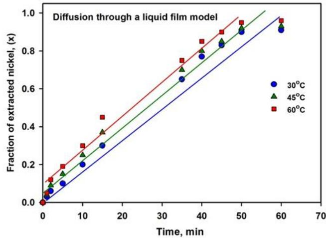
Figure 6. Fitting results by the diffusion through a liquid film model.
