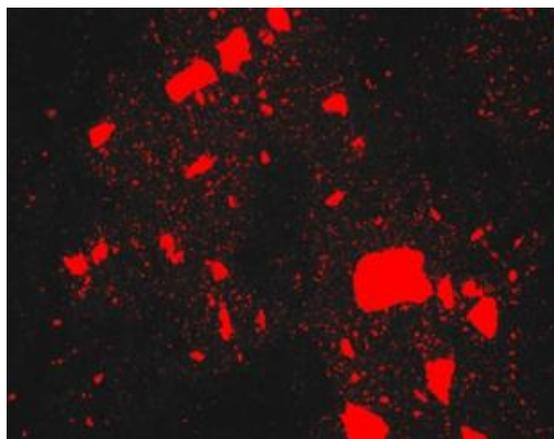
**Figure 11.** Transmission microscope image of the prepared iron nanoparticles.
