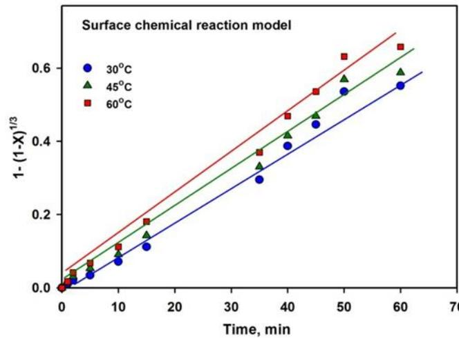
Figure 7. Fitting results by the surface chemical reaction model.
