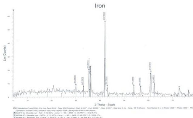
**Figure 1.** XRD analysis of mill scale sample.
