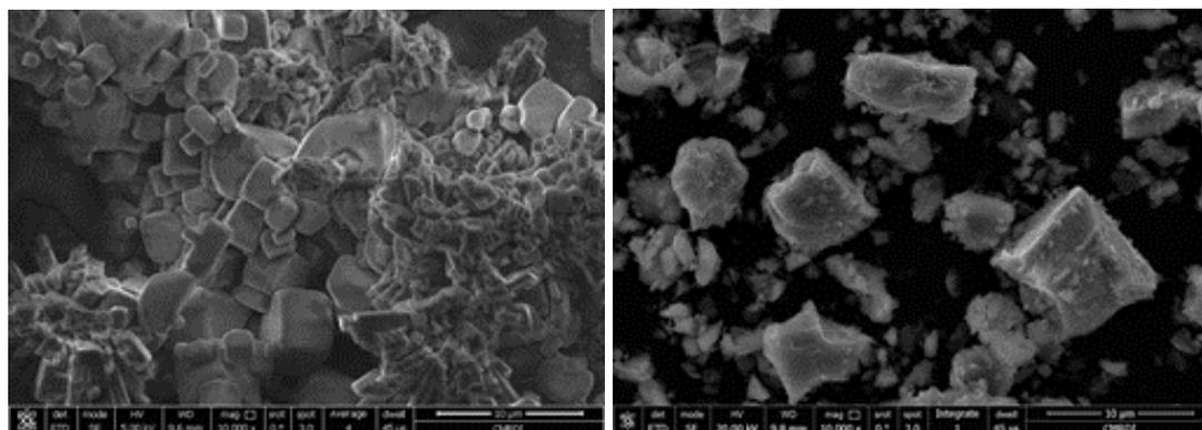
**Figure 10.** SEM images of the prepared iron nanoparticles.
