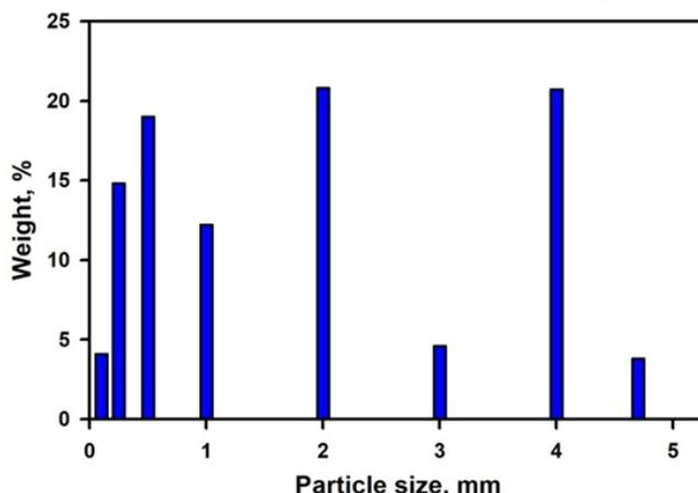
**Figure 2.** Sieve analysis of the crushed mill scale sample.
