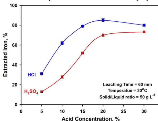
**Figure 3.** Effect of acid type and concentration on iron dissolution.
