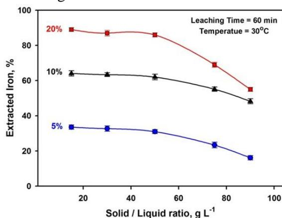
**Figure 4.** Effect of solid/liquid ratio on iron dissolution as a function of HCl concentration.
