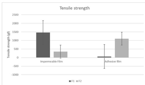
**Figure 3.** Rupture resistance of the impermeable (reservoir function) and adhesive films, comparing their respective formulations (1 and 2), (n=10).
