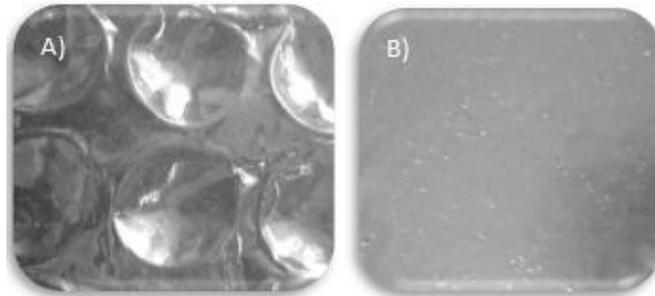
**Figure 10.** Layers that form the reservoir-like patch: A) Impermeable layer, B) Adhesive layer.
