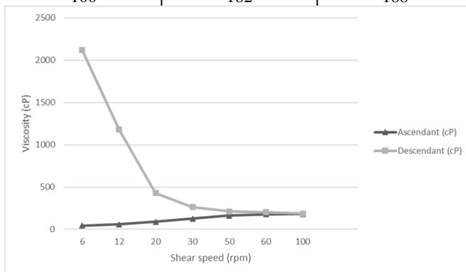
**Figure 5.** Relationship between the shear rate and viscosity of Pluronic-F127 gel with dexamethasone, ascendant, and descendant.
