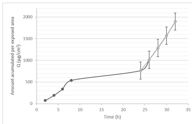
**Figure 9.** *In vivo* skin dexamethasone permeation profile of the reservoir-type transdermal patch.
