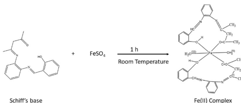
**Figure 1.** Schematic representation of reaction of Schiff's base with FeSO<sub>4</sub> to form Fe(II) complex at required reaction conditions.
