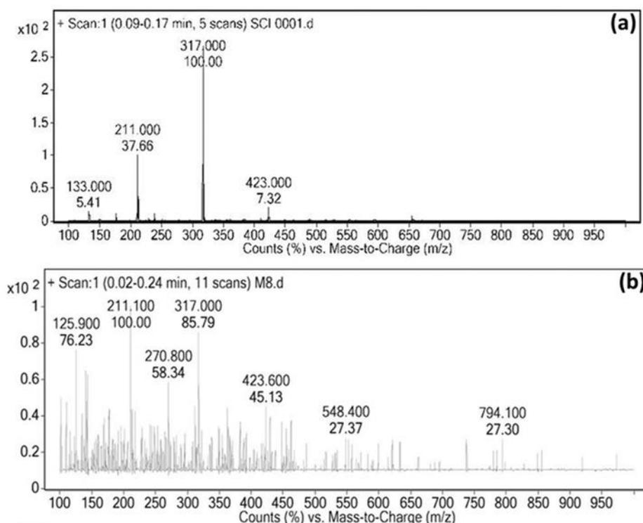
**Figure 4.** LC-MS Spectrum of (a) free Schiff's base [(Sal)(OPD) (AA)] and (b) [(Fe)(SAL)<sub>2</sub>(OPD)<sub>2</sub>(AA)<sub>2</sub>(H<sub>2</sub>O)<sub>2</sub>].H<sub>2</sub>O.(SO<sub>4</sub>)<sub>2</sub>.
