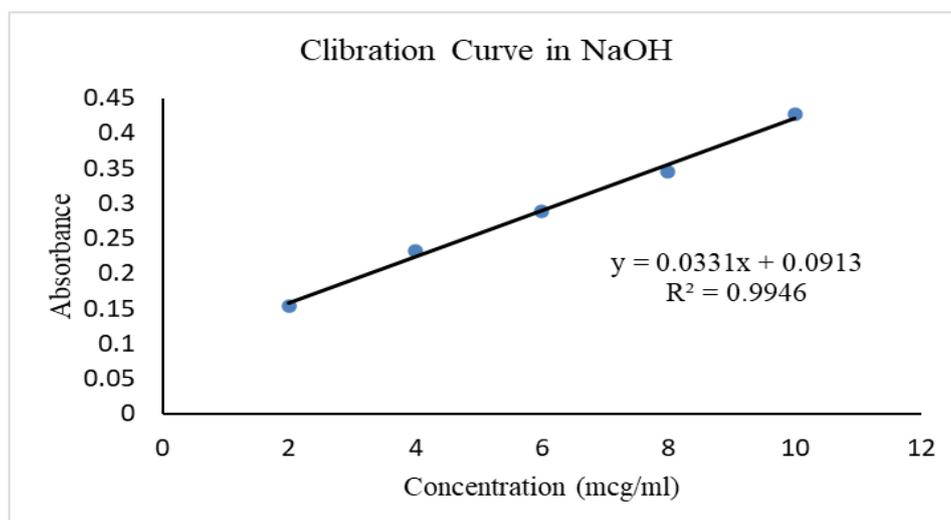
Figure 2. Calibration curve of hesperidin in 0.1 N NaOH.
