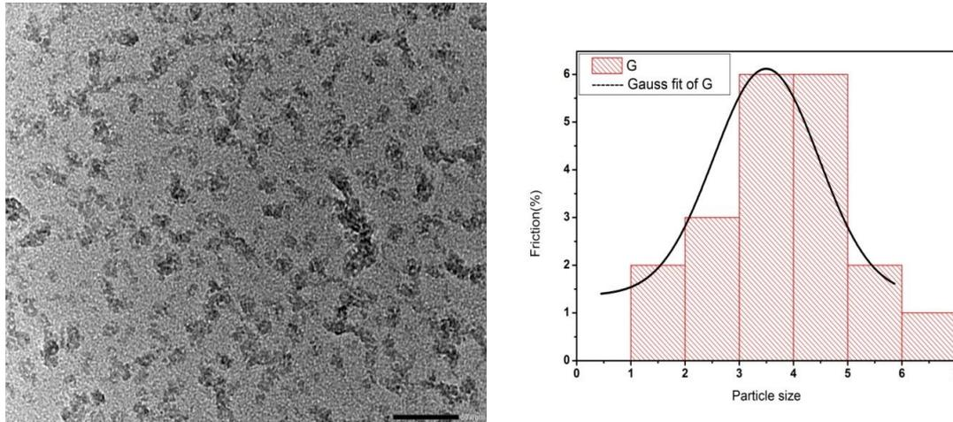
**Figure 2.** TEM image of ZnS nanoparticles and particle size distribution of ZnS nanoparticles.
