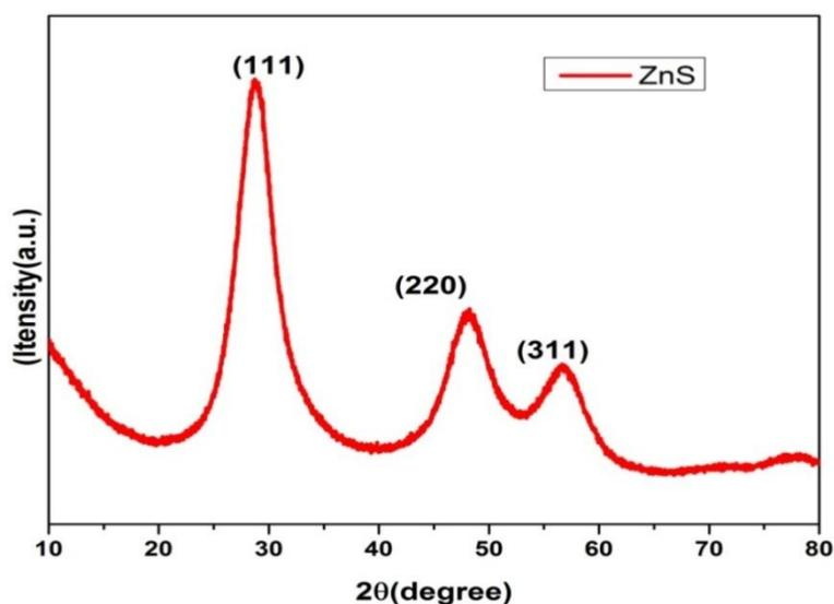
Figure 1. X-ray diffraction of ZnS nanoparticles.
