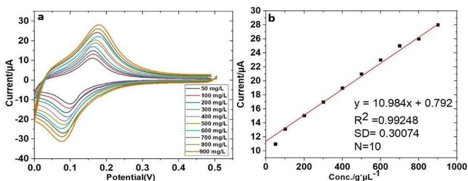
**Figure 3.** (a) CV plots of  $\beta$ -D glucose (50 –900 mg/L) in buffer solution (pH 5.2) on graphene electrode at  $100 \text{ mVs}^{-1}$  scan rate and (b) Calibration curve of response current ( $I/\mu\text{A}$ ) vs.  $\beta$ -D glucose concentration ( $\text{conc.}/\text{g.}\mu\text{L}^{-1}$ ).
