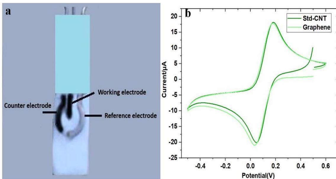
**Figure 1.** (a) Image of fabricated graphene electrode towards the detection of glucose under non-enzymatic conditions, (b) CV plots of 0.1 mol/L  $[\text{K}_3\text{Fe}(\text{CN})_6]$  in ammonium acetate buffer solution at  $100 \text{ mVs}^{-1}$  on the screen-printed std-CNT and prepared graphene electrode.
