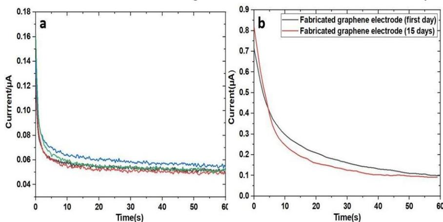
**Figure 5.** (a) Repeatability and (b) stability of fabricated graphene electrode.
