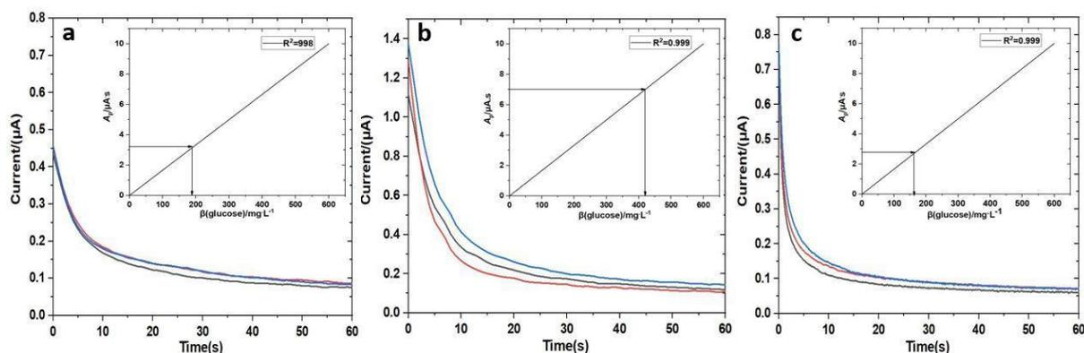
**Figure 4.** Amperometric curves of (a) apple juice, (b) coco-cola, and (c) honey in a PBS solution along with a calibration curve with a peak area vs. glucose concentration.
