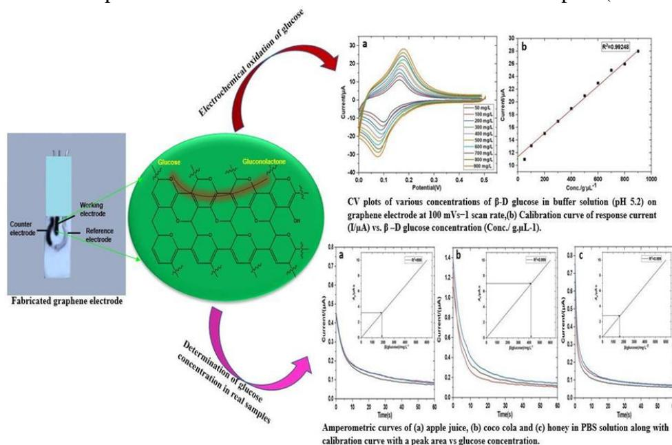
**Scheme 1.** Graphical abstract of electrochemical oxidation of glucose at fabricated graphene electrode.
