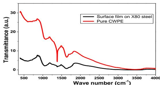
**Figure 5.** FTIR spectra of pure CWPE (black) and surface adsorbed film on X80 steel.
