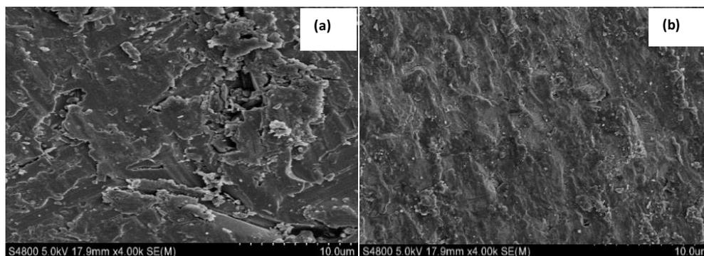
**Figure 6.** SEM micrographs of X80 steel surface immersed in (a) 1 M HCl and (b) 1 M HCl containing 1000 ppm CWPE.
