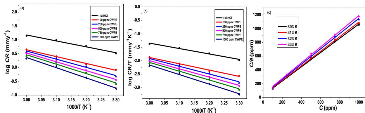
**Figure 4.** (a) Arrhenius plot and (b) Transition state plot, and (c) Langmuir adsorption isotherm for the inhibition of X80 steel corrosion in 1 M HCl using different concentrations of CWPE at 303 – 333 K.
