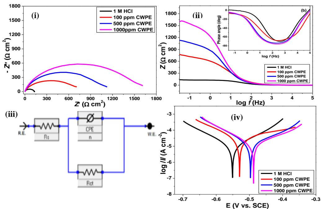
**Figure 2.** (i) Nyquist plot and (ii) Bode modulus and phase angle plot (iii) Equivalent circuit model and (iv) Potentiodynamic polarization curves for the corrosion of X80 steel in blank 1 M HCl and CWPE inhibited 1 M HCl.
