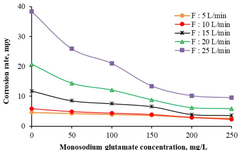
**Figure 2.** Effect of monosodium glutamate concentration on carbon steel corrosion rate in crude oil.
