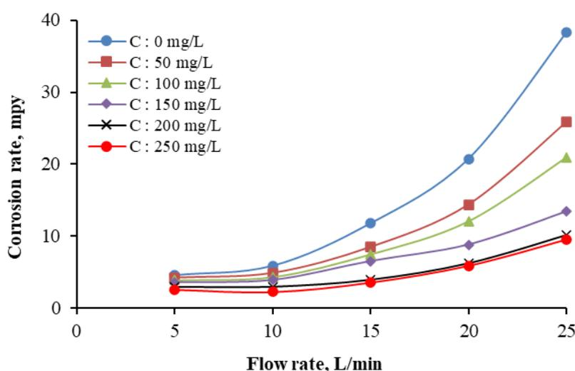
**Figure 1.** The influence of flow rate on the corrosion rate of carbon steel in a crude oil environment.
