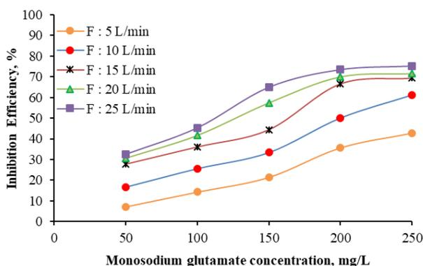
**Figure 3.** Monosodium glutamate's inhibitory effect on carbon steel in a crude oil environment.
