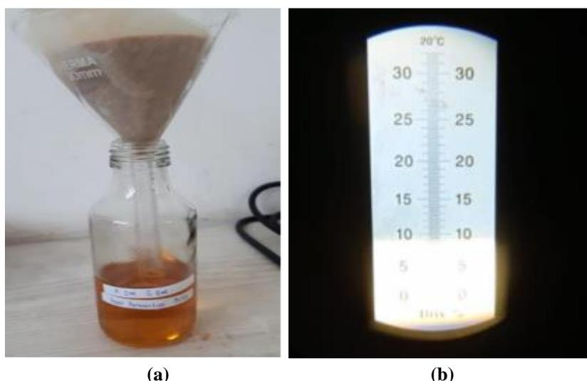
**Figure 2.** (a) The resulting product of enzymatic hydrolysis; (b) Glucose concentration measurement using Brix refractometer.
