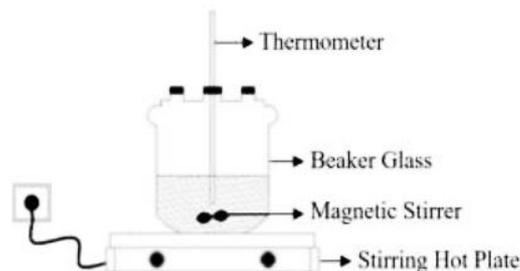
**Figure 1.** The schematic of a batch reactor for enzymatic hydrolysis process.
