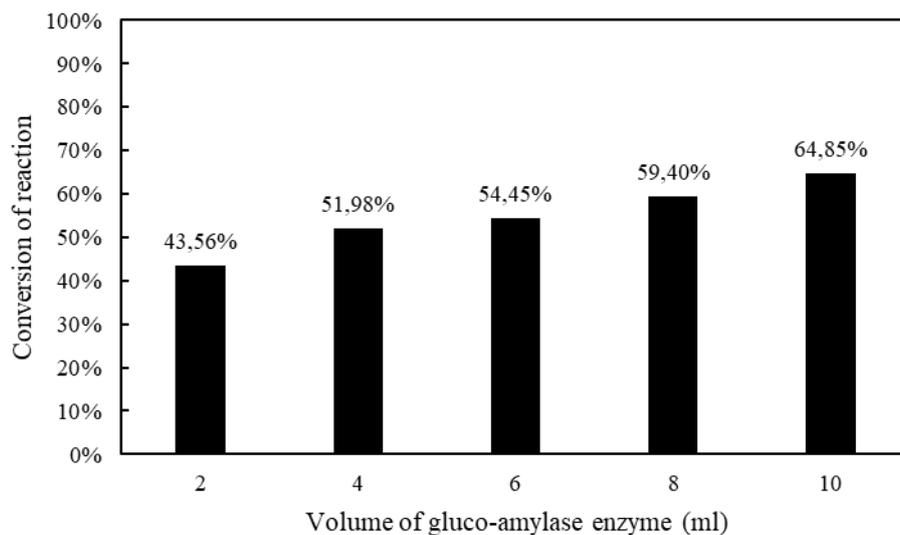
**Figure 4.** Conversion of hydrolysis with the variation of glucoamylase volume (ml) and fixed  $\alpha$ -amylase volume at 10 ml.
