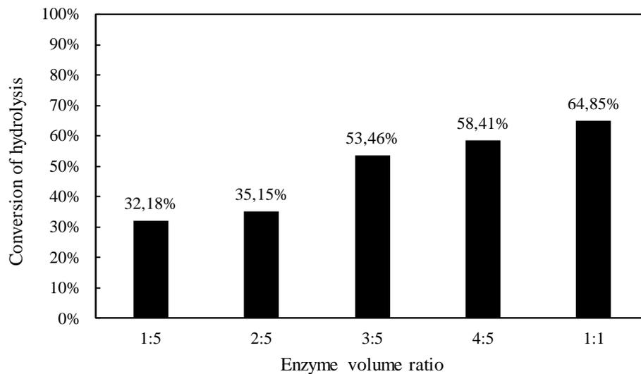
**Figure 3.** The effect of enzyme volume ratio with glucoamylase volume was fixed at 10 ml towards the conversion of enzymatic hydrolysis.
