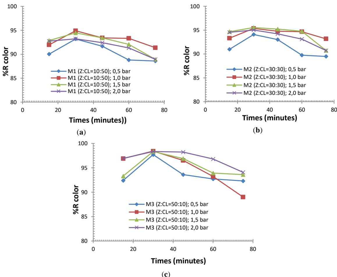
**Figure 4.** Effect of time of cross-flow filtration system on color rejection coefficient at various pressure variations for (a) M1 membrane; (b) M2 membrane; and (c) M3 membrane.
