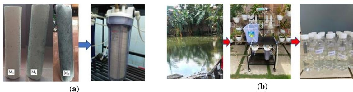
**Figure 6.** The membrane products and permeate flow water as (a) M1, M2, and M3 membranes, and the housing that already contains the M3 membrane; (b).
