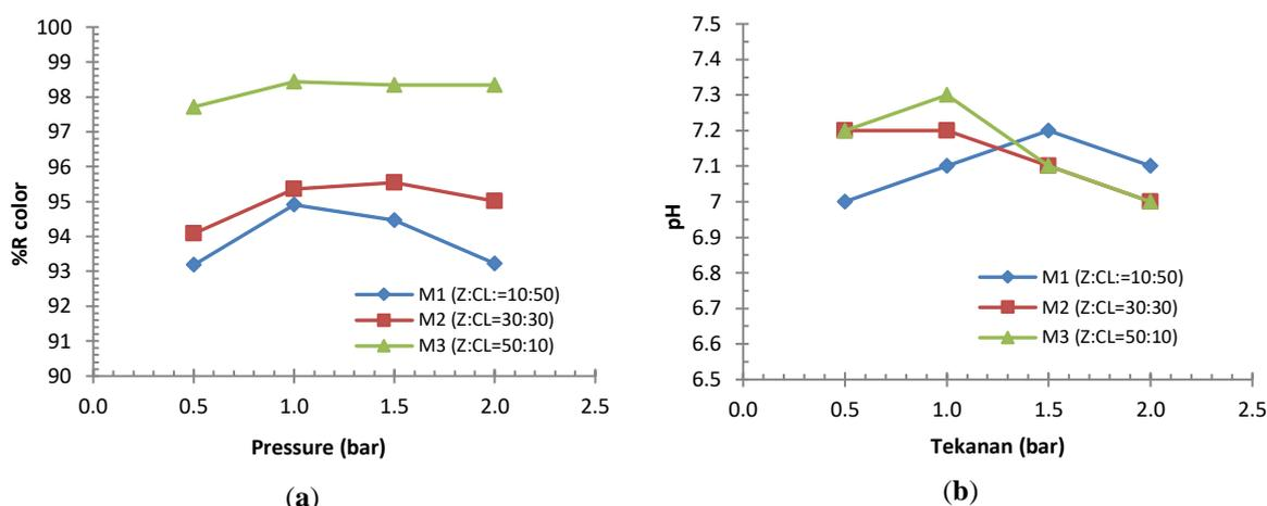
**Figure 5.** Effect of operating pressure on variations in membrane composition on (a) the rejection coefficient of peat watercolor, (b) pH of peat water.
