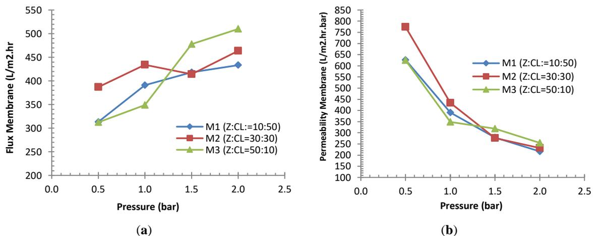
Figure 3. Effect of pressure on various membrane composition variations on (a) membrane flux, (b) permeability membrane.
