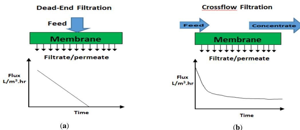
**Figure 1.** Membrane operating systems as: (a) dead-end filtration; (b) cross-flow filtration.
