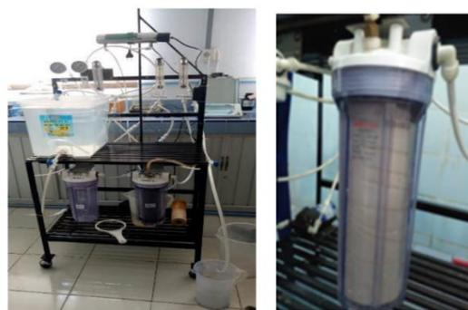
**Figure 2.** Prototype of unit tubular ceramic membrane microfiltration process [5] as (a) schema prototype; (b) unit process; (c) housing membrane.
