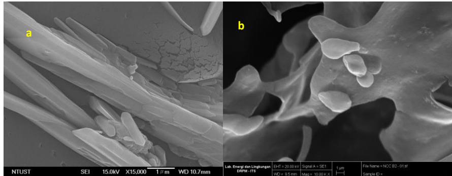
Figure 2. SEM images of (a) CNC; (b) CNC-chitosan hydrogel.
