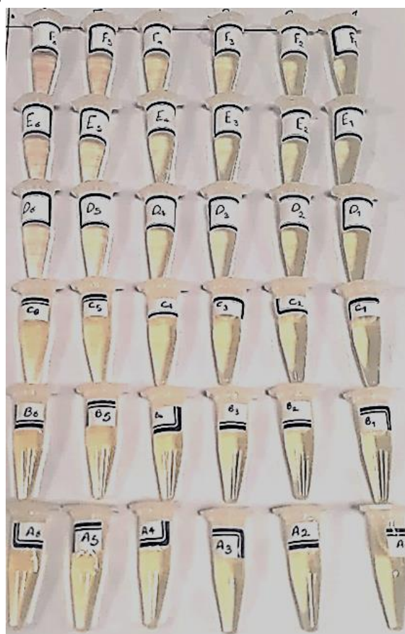
Figure 2. Visual changes in Aloe vera gel color reacting with various concentrations of H_2O_2
