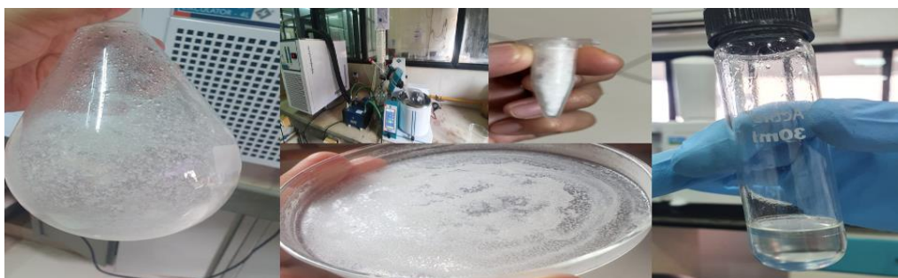
Figure 6. Extracted lipid sample collection after the Bligh and Dyer method by evaporation using Rota evaporator and FAME formation for gas chromatography and mass spectrometry.
