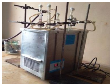
Figure 6. Ultrasonication with a condenser.
