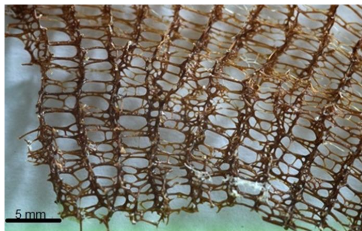
Figure 8. Acellular flat skeletal chitinous scaffold isolated from I. basta demosponge.
