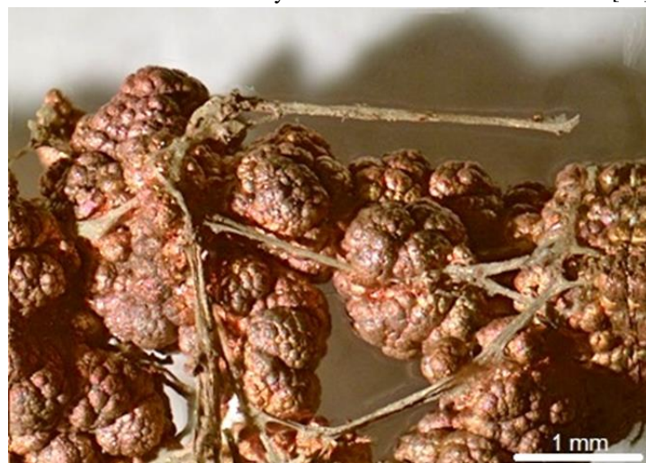
Figure 13. Metallization of 3D chitinous matrix isolated from A. fulva demersponge using electroplating of copper.
