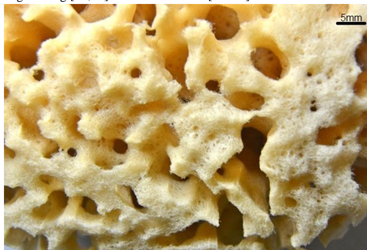
Figure 2. Typical example of 3D spongin scaffold isolated from marine demosponge Hippospongia communis . This biological material possesses a well-developed surface due to the existence of both micro- and macropores.
