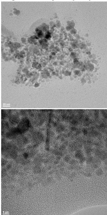
Figure 4: TEM images of magnetic nanofluid
