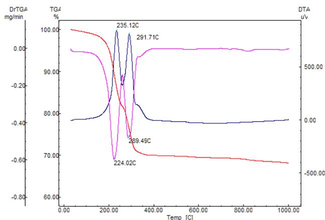
Figure 2: Thermal analysis of  $\text{Fe}_3\text{O}_4@\text{C}_{14}$
