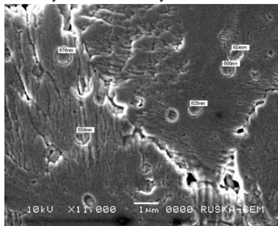
**Figure 2:** SEM image of Copper nanoparticles formed by *Aspergillus species* 3800X.
