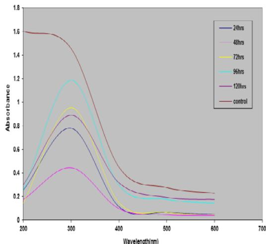
**Figure 1:** UV-Vis spectrum of aqueous medium during synthesis of copper nanoparticles
