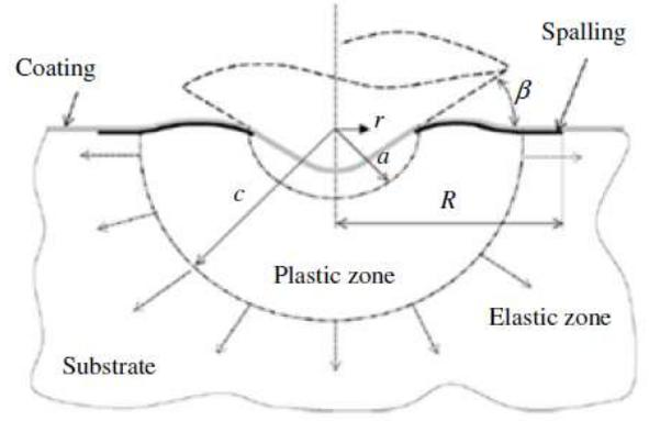
**Figure 2.** Schematic indentation by an axisymmetric indenter [14].
