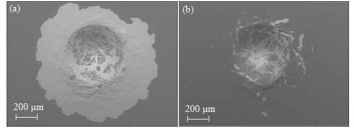
Figure 3. DLC spalling for an indentation load of 400 N: (a) Sample B; (b) Sample C.
