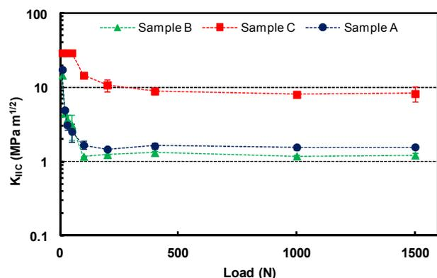
Figure 7. Interface fracture toughness.
