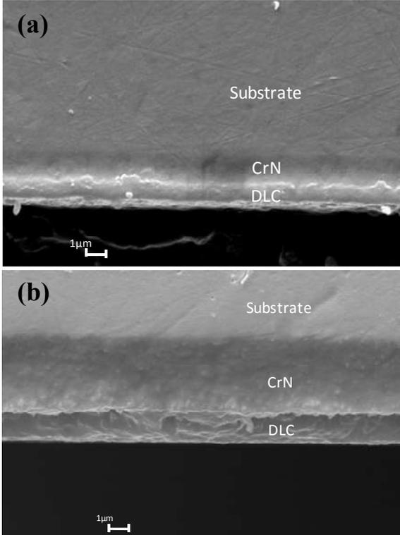
**Figure 1.** Cross sections of the coated systems:(a) Family 2; (b) Family 1.
