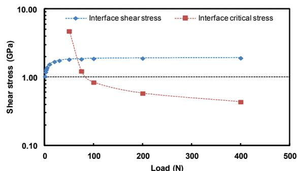
Figure 8. Example of critical interfacial stresses, obtained experimentally, and shear stresses at the interface, calculated by simulations, for the thinner coatings on sample C.
