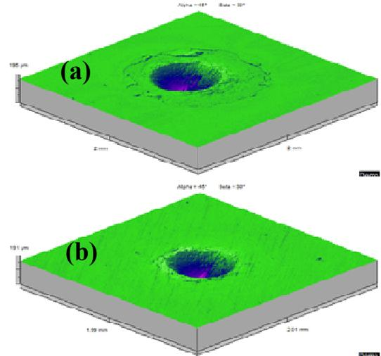
Figure 4. Laser interferometry images of DLC spalling for an indentation load of 400 N: (a) Sample B; (b) Sample C.
