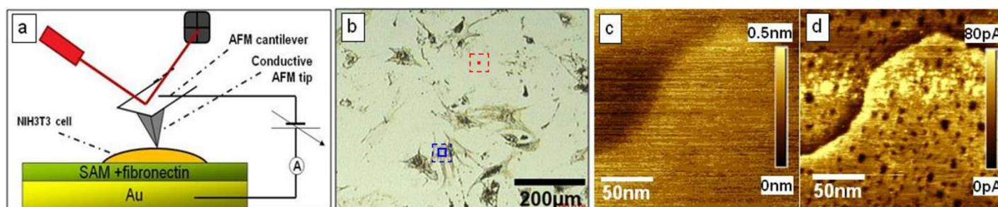
**Figure 1.** [a] Schematic diagram for imaging NIH3T3 cells by CAFM. [b] Bright-field optical image of the NIH 3T3 cells. CAFM topography [c] and current [d] images of a CHO(CH<sub>2</sub>)<sub>10</sub>S/Au(111) SAM under +1 V at ambient conditions at 1 Hz scan rate.
